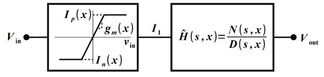
The circuit parameters,  $I_p$ ,  $I_n$ ,  $g_m$ , the poles and zeros in the transfer function are parameterized and estimated using neural network metamodels:
