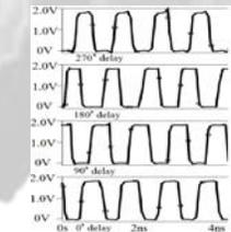
Four-Phase Source: Using Large Dimension Inverters to Construct Different Signals
