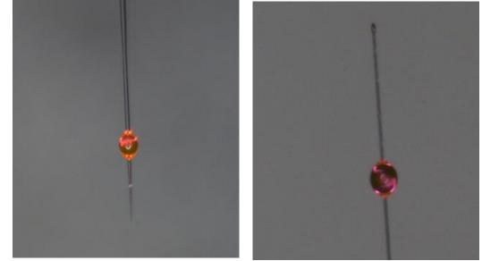
Fig.3: Photonic microresonators captured under the microscope.
