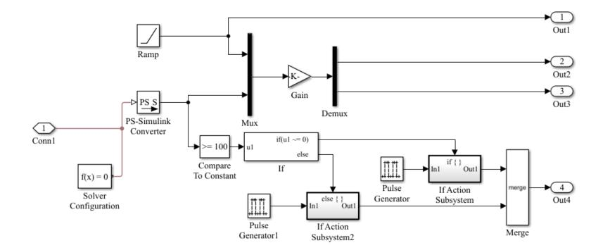
*Fig.7: Functional block of the photonic sensor model 2.*
