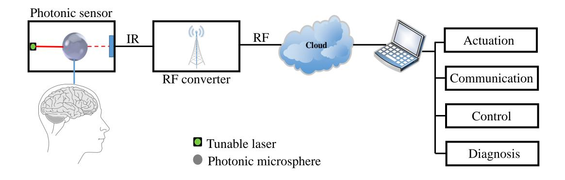
Fig.5: A conceptual BCI system based on photonic sensing.
