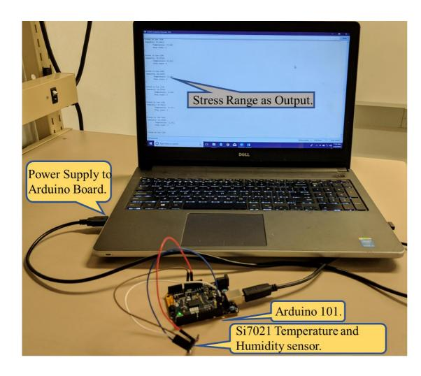
✤ An Adafruit Si7021 Temperature and Humidity Sensor along with Arduino/Genuino 101 were used.
