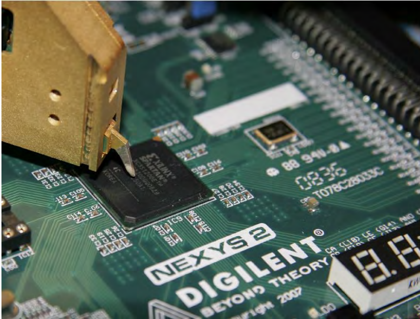
Langer ICR HH 150 probe over Xilinx Spartan3E-1200 FPGA
