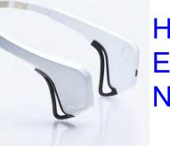
Headband with Embedded Neurosensors
