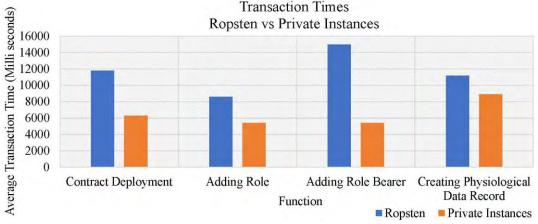
Transaction times of Private Ethereum in SaYoPillow is 2X faster in operations as compared to public ethereum test network Ropsten, as it is impacted by network congestion.
