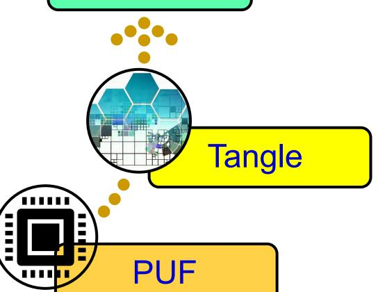
PUFchain 3.0 is the idea of integrating PUF with scalable Tangle DLT using MAM communication protocol by creating a MAM communication channel in Tangle using PUF key
