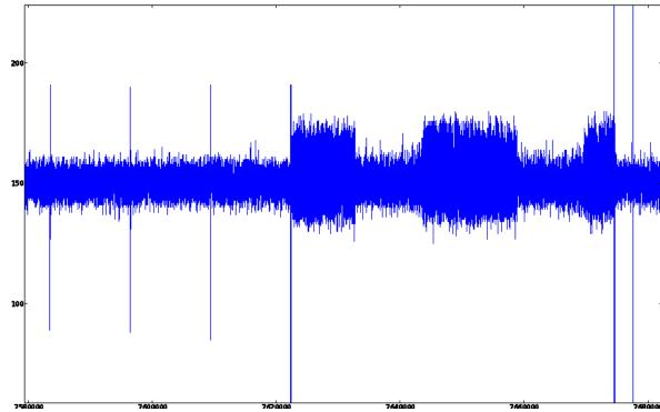
Magnification of the last part of the complete trace. Three trigger signals can be identified: (1) between oscillator phase and error correction phase, (2) between error correction and hashing, and (3) at the end of hashing.
