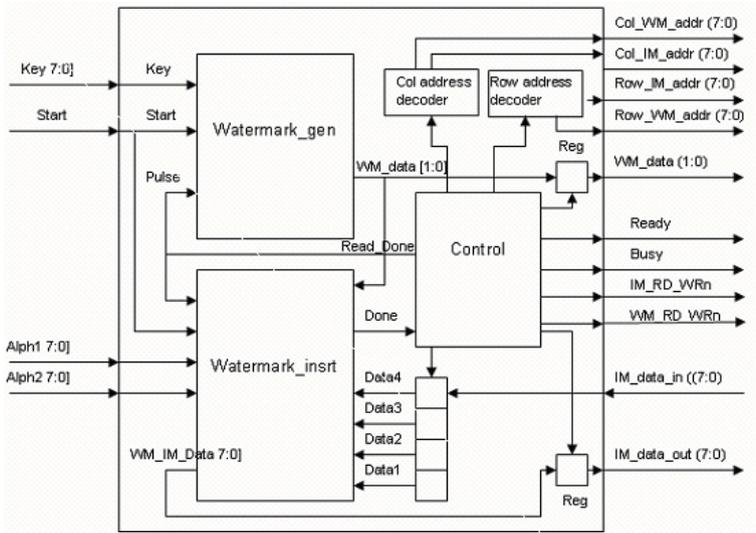
Fig. 1. Datapath and Controller for the Proposed Chip.
