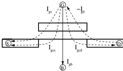
(a) Gate leakage current paths in a NMOS transistor
