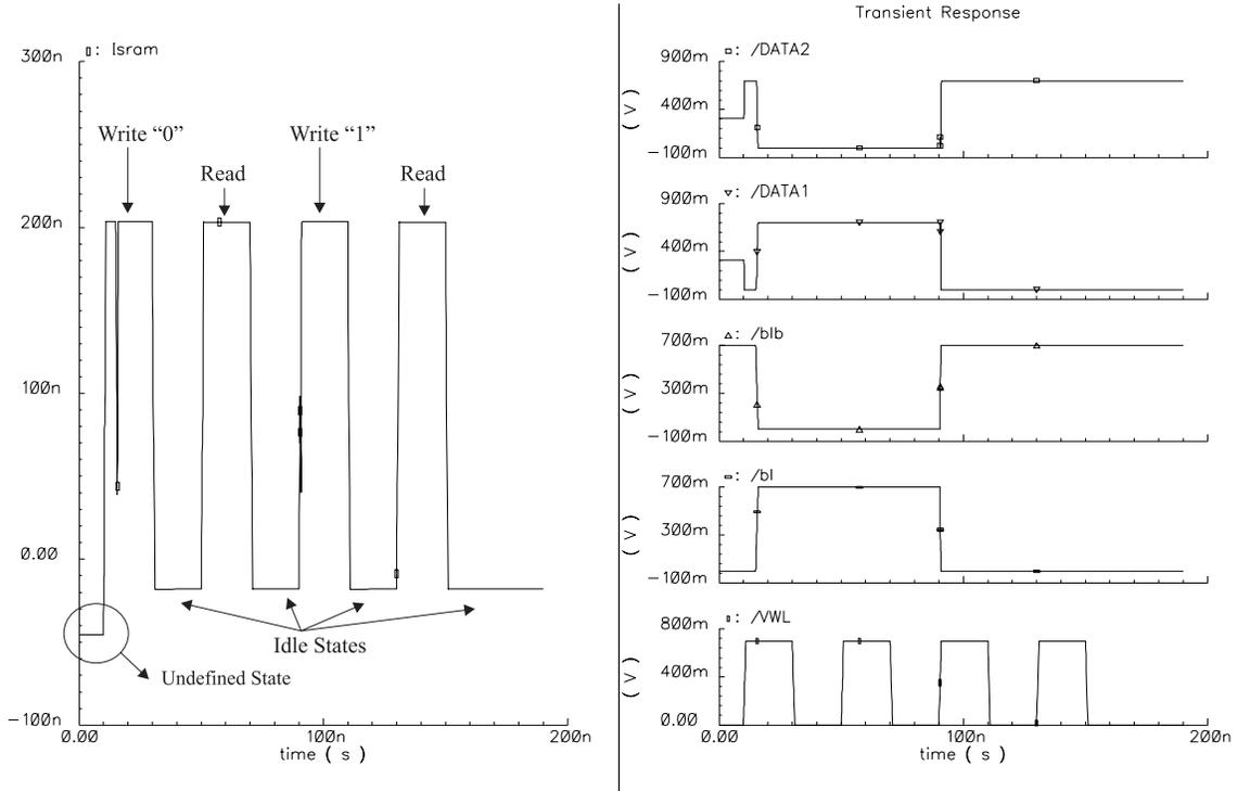
Figure 4: Plots representing simulation results from the input waveform and the corresponding gate leakage current in an SRAM cell
