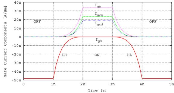
(b) Components of  $I_{ox}$  in NMOS corresponding to a pulse input
