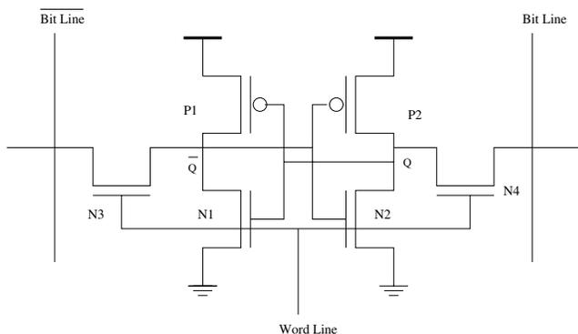
Figure 1: Basic diagram of a 6T SRAM cell.
