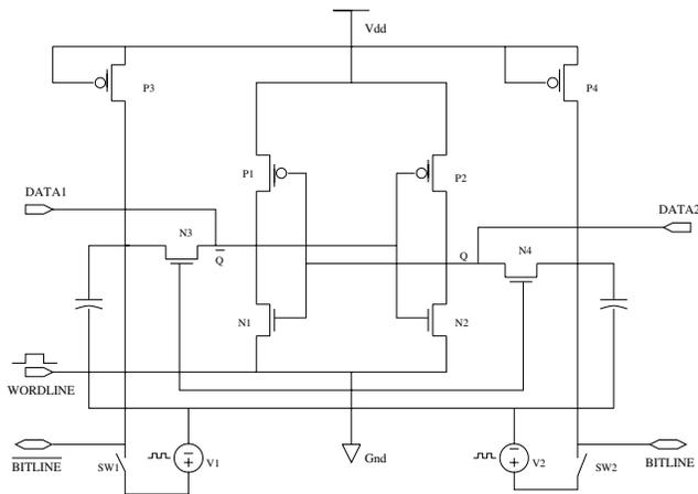
Figure 3: Testbench used for the analysis of the gate leakage in an SRAM based on circuit from [14]
