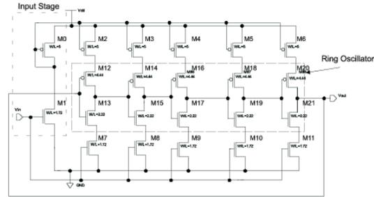
Figure 2: Transistor level diagram of the VCO.
