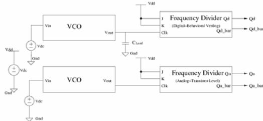
Figure 1: Block diagram of the VCO along with an analog frequency divider and a digital frequency divider. The role of the capacitor  $C_{Load}$  is to model capacitive loading effects, as explained in the text.
