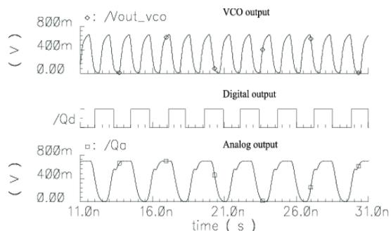
Figure 4: Output waveforms of the VCO, digital frequency divider, and analog frequency divider
