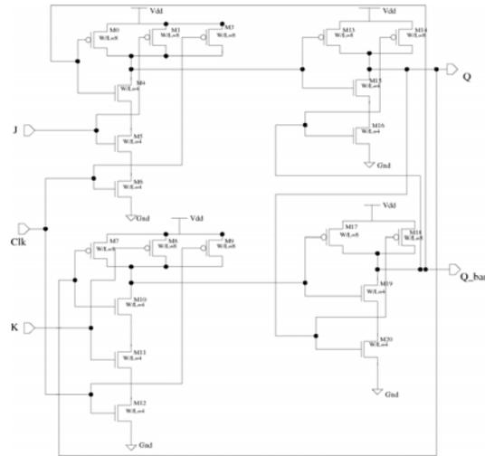
Figure 3: Transistor level diagram of the frequency divider.
