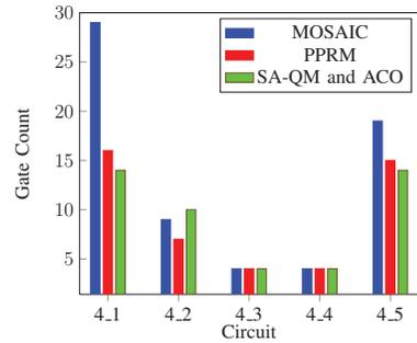
Fig. 4: Comparison Graph with MOSAIC and PPRM for  $4 \times 4$  circuits
