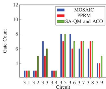
Fig. 3: Comparison Graph with MOSAIC and PPRM for  $3 \times 3$  circuits
