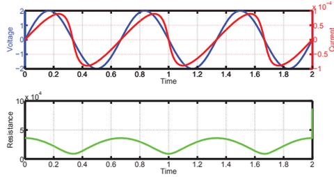
(a) Time-domain simulation result for a 2-V, 1.5 Hz applied sinusoidal voltage.
