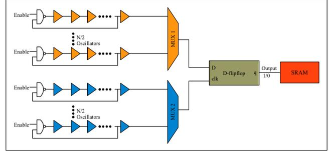
Fig. 5. Proposed Design of Power Optimized Inverter based MKG PUF.
