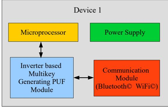
Fig. 3. Deployment of Inverter based Multi-key Generation PUF.
