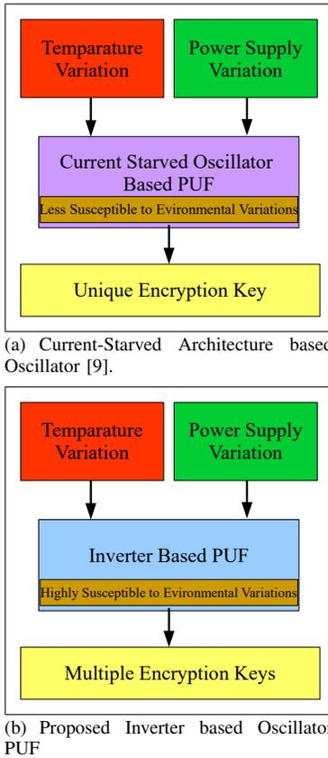
Fig. 2. Comparison of PUF Architectures.
