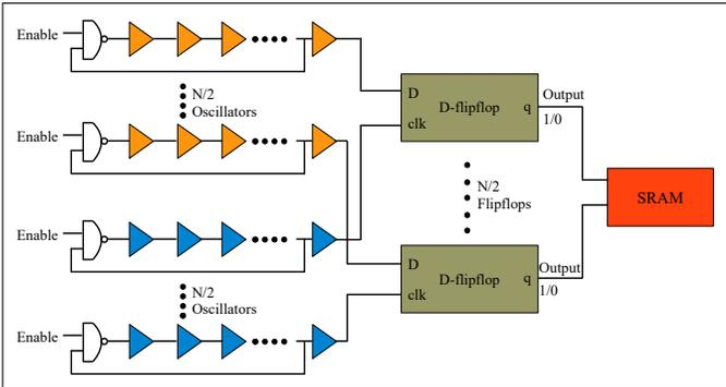
Fig. 4. Proposed Design of Speed Optimized Inverter based MKG PUF.
