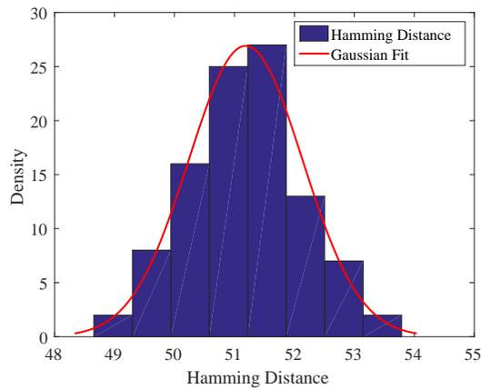
Fig. 9. Hamming Distance Power Optimized Inverter based MKG PUF.
