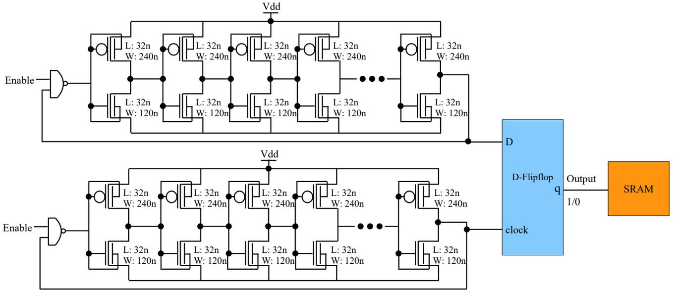
Fig. 6. Design of Inverter based MKG PUF.
