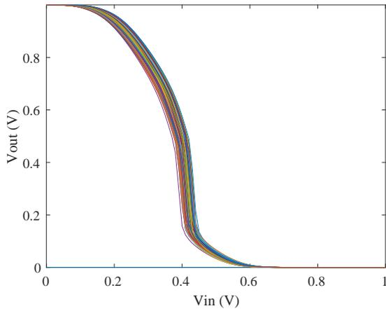
Fig. 7. DC Analysis of Inverter with Process and Mismatch Variations.
