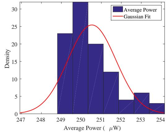
Fig. 12. Average Power of Speed Optimized Inverter based MKG PUF.
