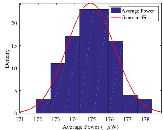
Fig. 13. Average Power of Power Optimized Inverter based MKG PUF.
