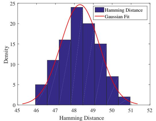
Fig. 8. Hamming Distance of Speed Optimized Inverter based MKG PUF.
