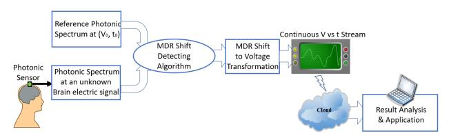
Figure 1: Proposed Photonic Brain-Computer Interface (BCI) Architecture
