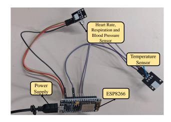
Fig. 7. Hardware Implementation of Smart-Steering
