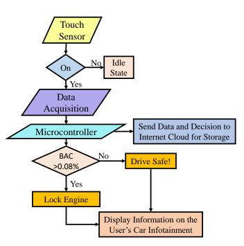
Fig. 5. Design Flow of Smart-Steering
