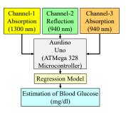
Fig. 2: Processing steps for the Proposed iGLU.
