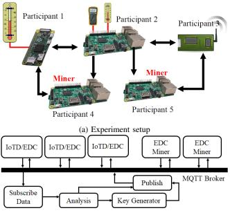
(b) Real-time system implementation architecture.Fig. 6: Experiment setup and implementation architecture of
