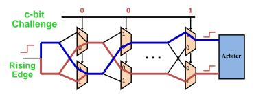
Fig. 2. Physical Unclonable Function
