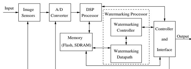
Fig. 2. System Architecture of a Secure Digital Still Camera
