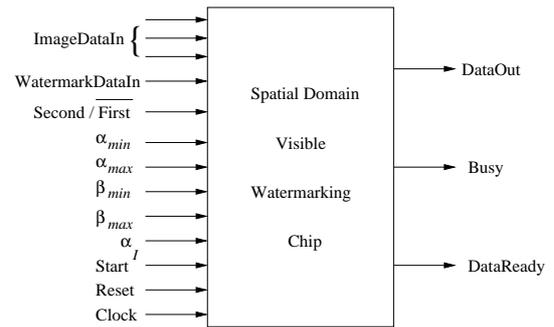
Fig. 7. Pin diagram for the Proposed Watermarking Chip
