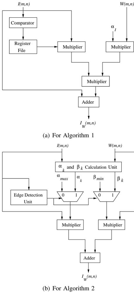
Fig. 3. Datapath Architectures for the Visible Watermarking Algorithms
