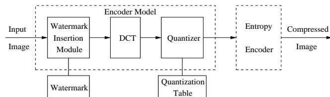
Fig. 1. Block Level View of a Secure JPEG encoder [6]
