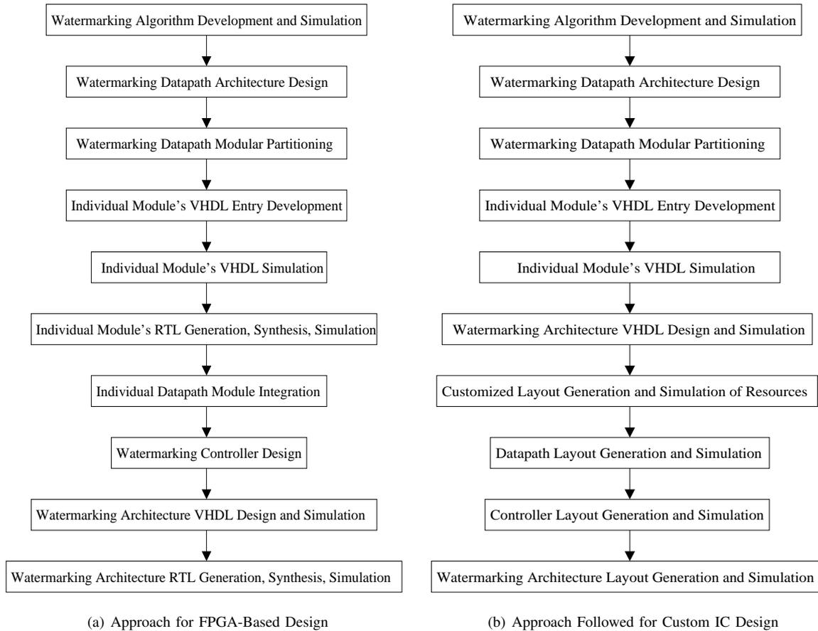
Fig. 6. Design Flow Followed for the FPGA-Based Prototyping and Custom IC Design
