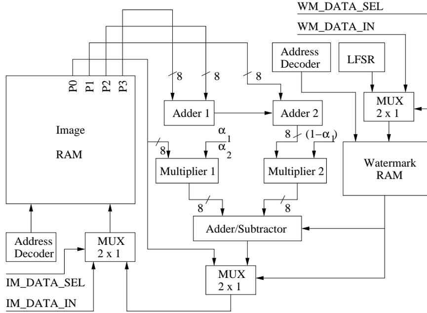
Fig. 3. Datapath for Invisible Robust Watermarking
