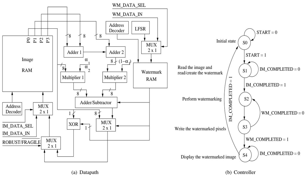
Fig. 5. Datapath and Controller for the Architecture of the Chip that Can Perform Both Invisible Robust and Invisible Fragile Watermarking in the Spatial Domain
