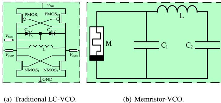
Figure 9: Circuits of analog oscillators.
