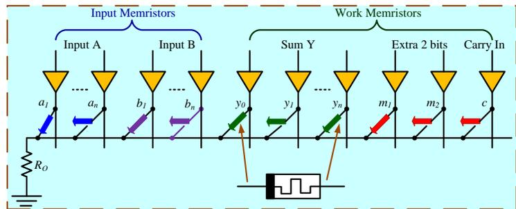
Figure 10: A memristor-based  $n$ -bit adder.
