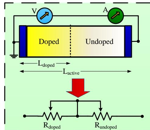
Figure 6: Memristor biasing.
