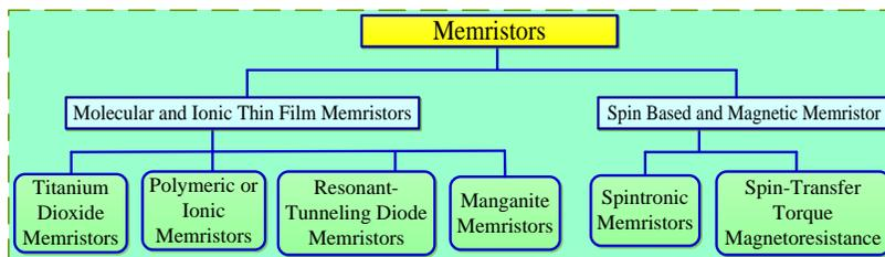
Figure 3: Different types of memristors.
