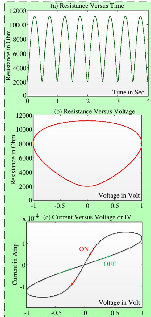
Figure 7: Characteristics of a memristor.
