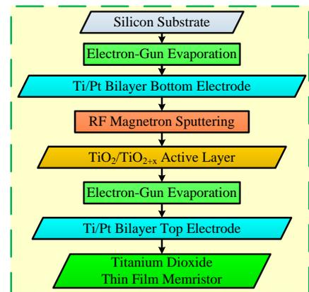
Figure 5: Memristor fabrication.
