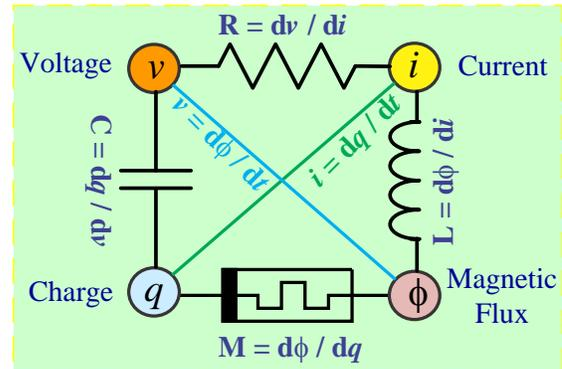
Figure 2: Memristor directly relates magnetic flux and charge; the missing connection among the 4 variables,  $v$ ,  $i$ ,  $q$ , and  $\phi$ .
