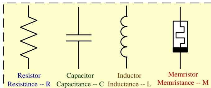
Figure 1: Memristor: The 4th Fundamental Element.
