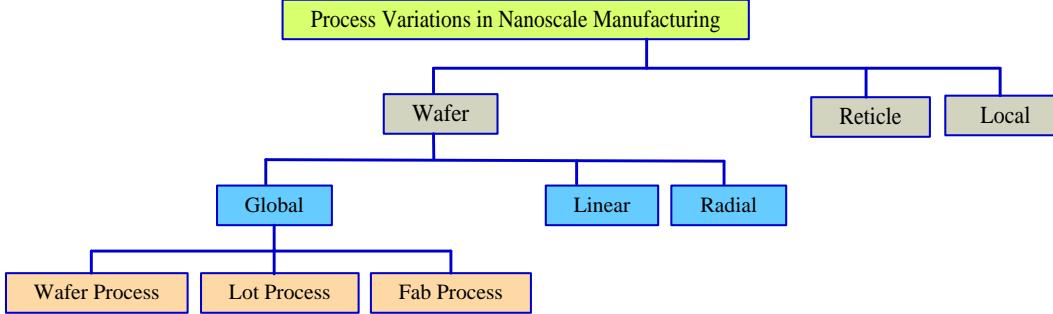
Figure 5: Types of process variations in nanoscale technology.
