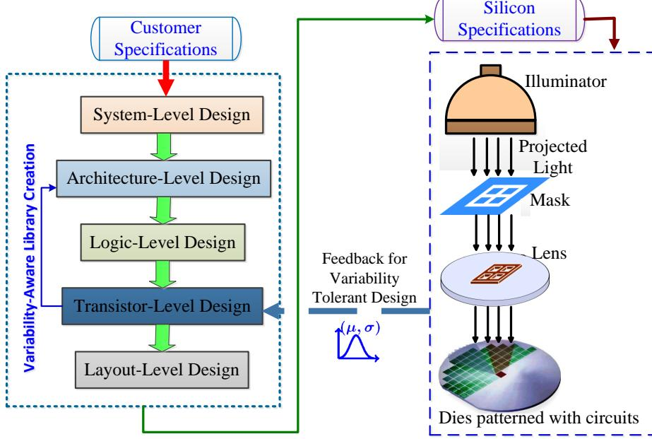
Figure 9: The key idea is to incorporate the process variation effects during architectural-level design flow.
