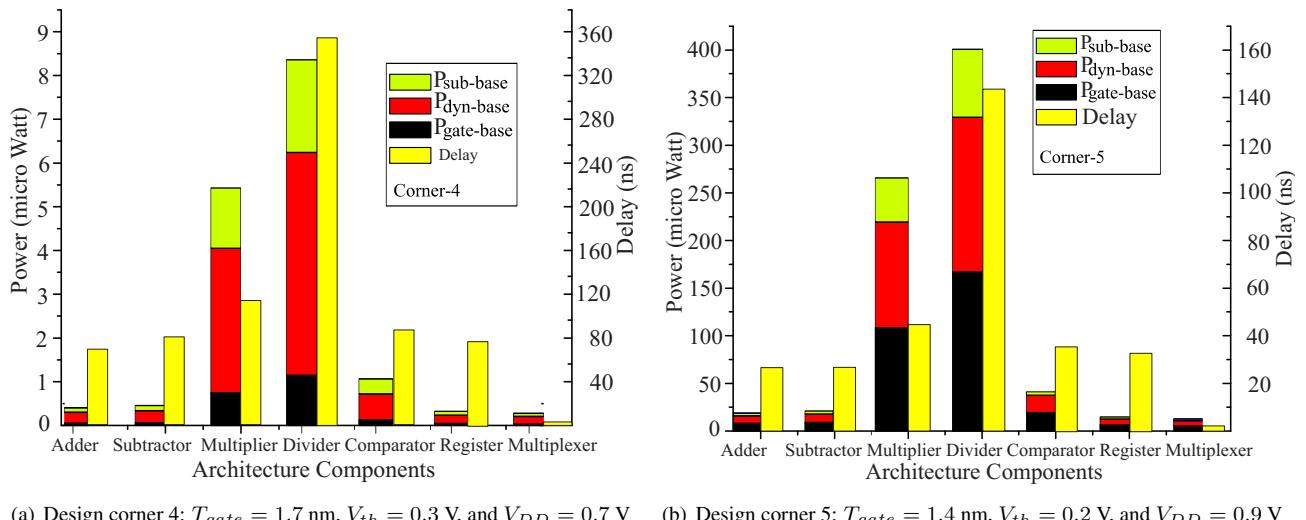
Figure 14: Nominal results showing individual components of power consumption for different output corners (corner 5 and corner 4).
