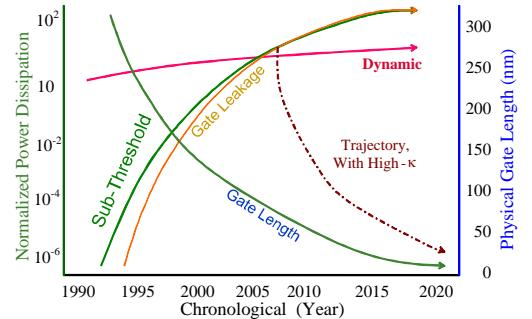
Figure 2: Prediction of trends of major sources of power dissipation in nanoscale chips.
