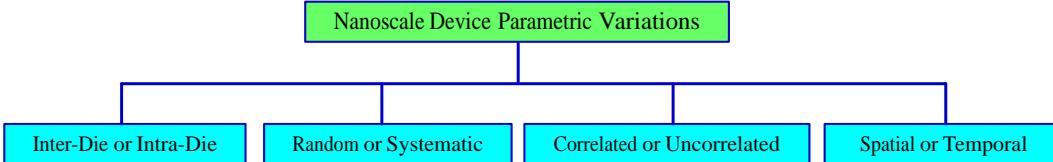
Figure 6: Classification of different types of process variation in nanoscale technology for modeling during the design phase.
