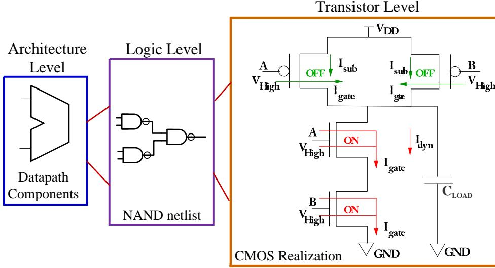
Figure 12: Three levels of abstraction in which datapath components are realized using 2-input NAND gates. The transistor level diagram shows worst-case tunneling current paths in the constituent NAND gates. The worst-case occurs when both inputs are high, i.e.,  $A = B = V_{High}$ .
