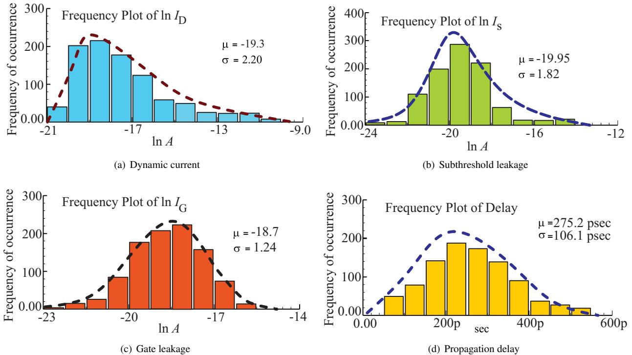
Figure 15: Effects of statistical process variation on dynamic, subthreshold-leakage and gate-oxide leakage current, and delay in a 2-input NAND gate.
