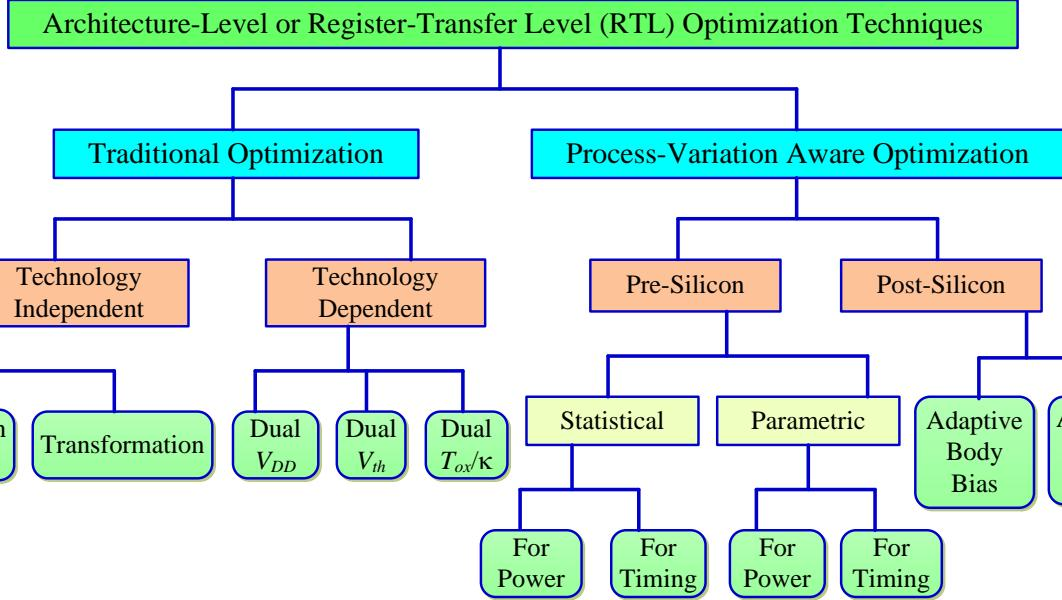
Figure 8: Overview of Architecture Level Optimization Techniques.
