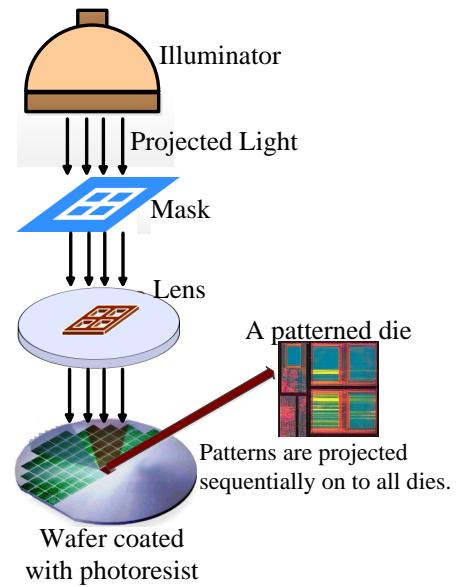
Figure 4: Broad perspective of the lithographic process. The patterns are projected sequentially onto all dies on the wafer, printing the desired circuit on the dies, one after another.
