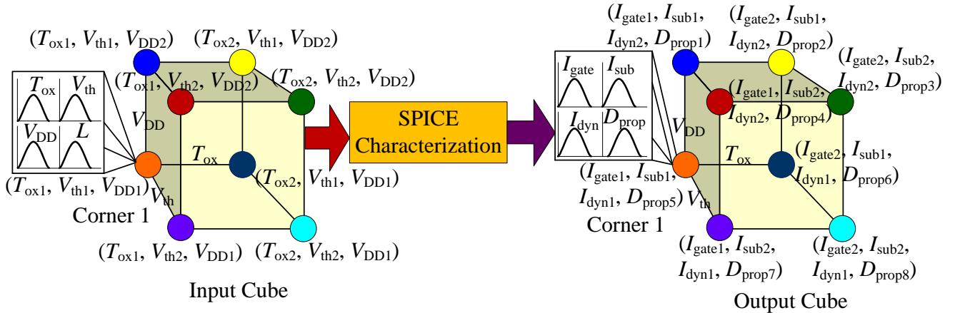
Figure 13: Monte Carlo simulation methodology to account for physical process variations and power supply variation in the power and performance of circuits. Corner 1 is assumed as the baseline corner.
