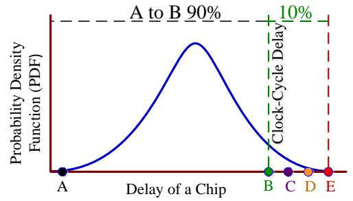
Figure 10: The concept of tradeoff in the statistical approach: the delay values of datapath components as a function of timing yield. A similar analogy can be used for power yield.
