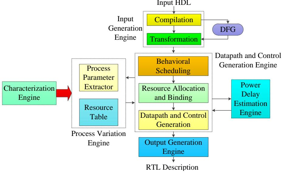
Figure 11: The proposed statistical behavioral synthesis framework for process variation aware design space exploration.
