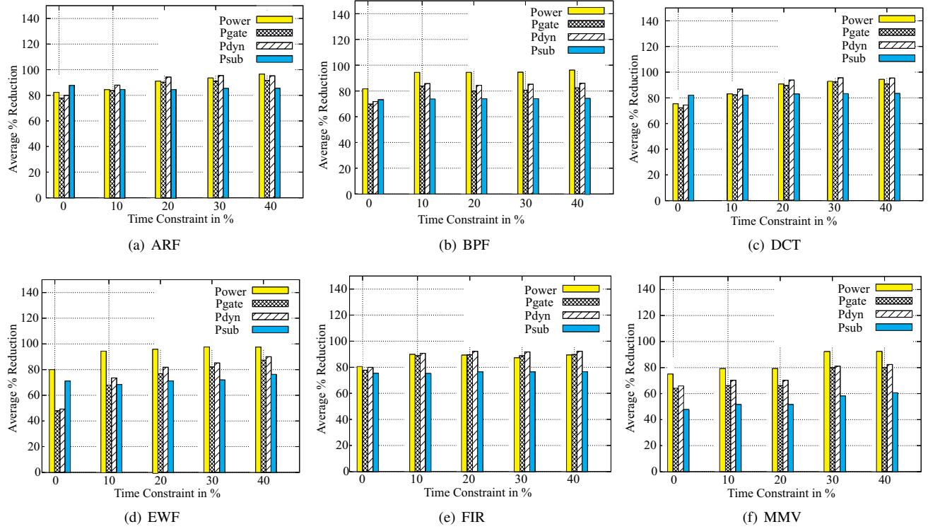
Figure 16: Experimental results showing the percentage reduction in various leakage and dynamic power components for selected benchmarks. The X-axis represents various time constraints as percentage and the Y-axis represents percentage reduction. For each time constraint, the data is averaged for various resource constraints.
