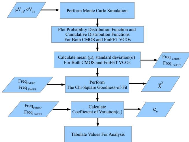
Fig. 7. Flow of process variation analysis of the FinFET VCO.
