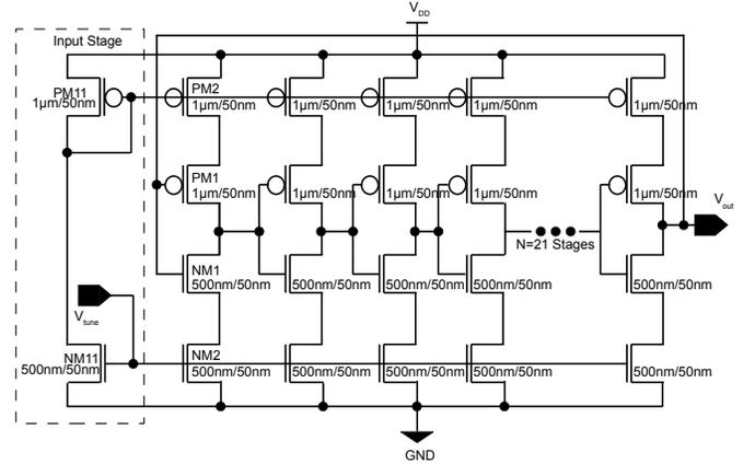
Fig. 3. Schematic diagram of a 45nm CMOS VCO circuit.
