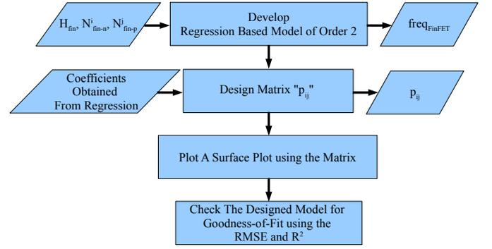
Fig. 9. Flow of proposed width quantization aware modeling of FinFET VCO.
