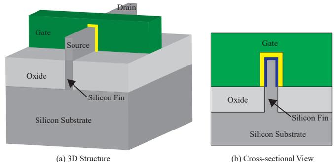
Fig. 1. Structure of Intel's tri-gate FinFET [6].
