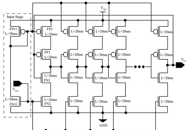
Fig. 4. Schematic diagram of a 15nm FinFET based VCO circuit.
