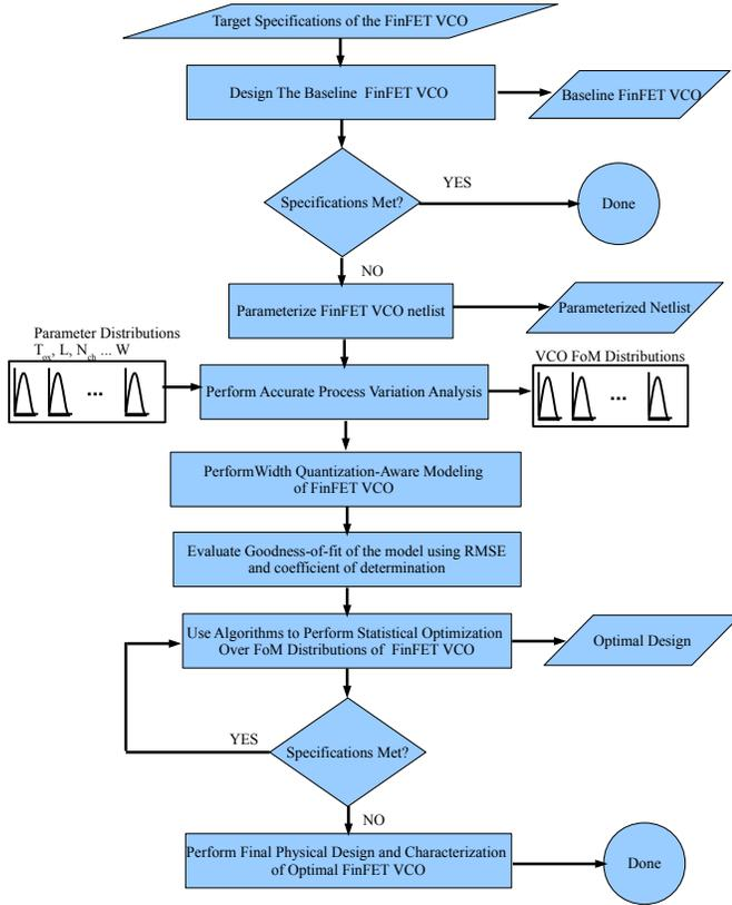
Fig. 2. Proposed methodology for FinFET based VCO.
