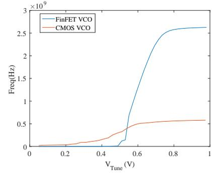
Fig. 6. Tuning curves of CMOS and FinFET VCOs.
