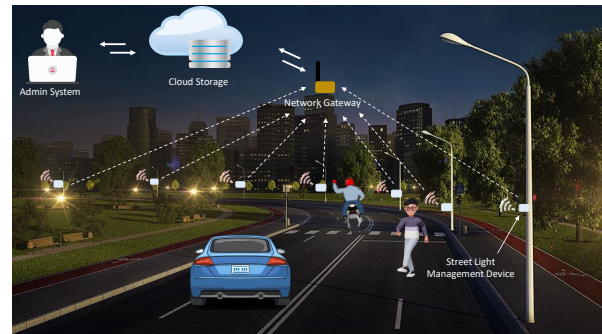
Fig. 1. Framework of smart street light management system
