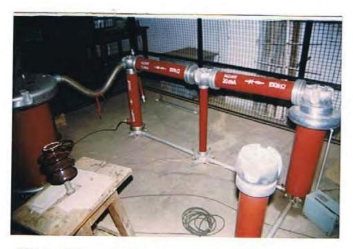
FIG. 2. EXPERIMENTAL SET UP FOR DC CORONA
