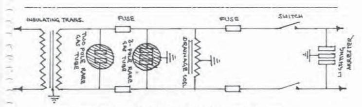
FIG.6. PROTECTIVE SYSTEM FOR COMMUNICATION CIRCUIT
