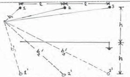
FIG. 2 THREE-PHAGE SYSTEM WITH THE ARRAY OF CONDUCTORS BUNDLED TOGETHER IN THEIR RESPECTIVE PHASES.
