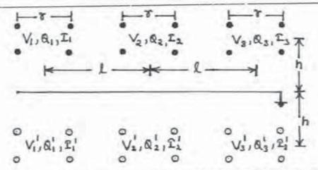
FIG.1 SCHEMATIC REPRESENTATION OF A THREE-PHASE EHV SYSTEM WITH IMAGE ARRAYS.
