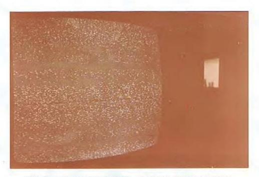
FIG. 6. TV INTERFERENCE IN CASE OF AC CORONA
