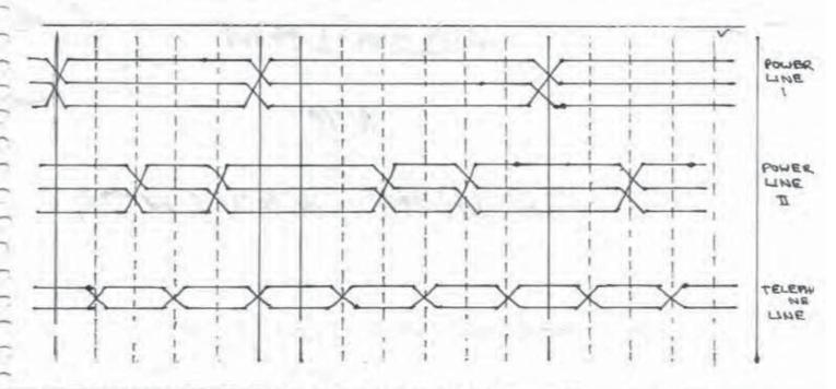
FIG.4 TRANSPOSITION SCHEME FOR TWO POWER LINES & A TELEPHONE LINE
