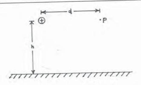
FIG. 1 SINGLE WIRE HVDC TRANSMISSION LINE
