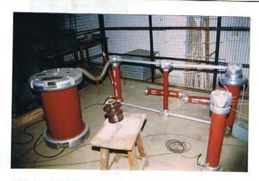
FIG.1. EXPERIMENTAL SET UP FOR AC CORONA
