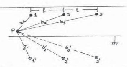
FIG.3. THREE PHASE SYSTEM WITH THE ARRAY OF CONDUCTORS BANDED TOGETHER IN THEIR RESPECTIVE PHASES.
