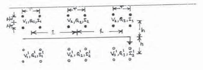
FIG1.SCHEMATIC REPRESENTATION OF A THREE PHASE EHV SYSTEM WITH IMAGE ARRAYS.
