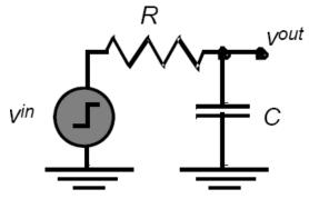
Find the transient response of the circuit for output voltage using LTSpice. What is the time to reach 50% point? What is the time to reach 90% point?
