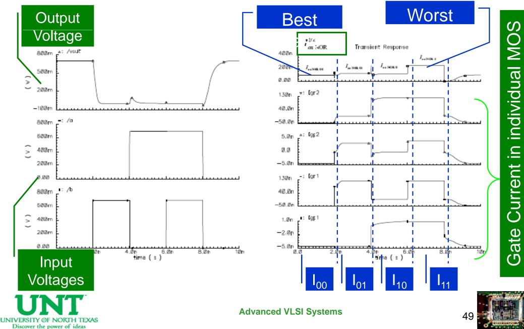
Gate Leakage in Logic Gate (Transient Study)
