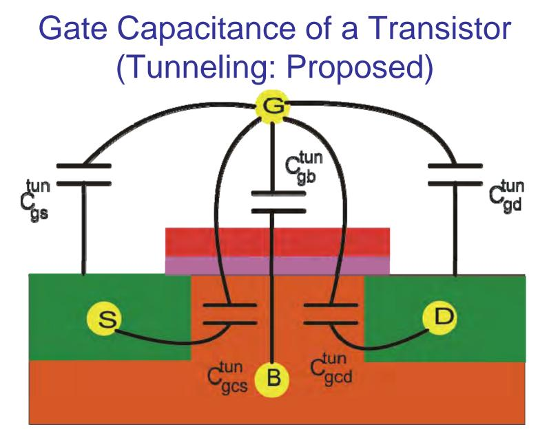
We propose that transient in gate tunneling current due to state transitions are manifested as capacitances.
