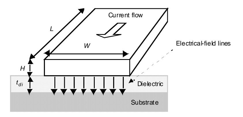
• When the width of the wire is substantially larger than thickness of the insulating material, the total capacitance of the wire:
