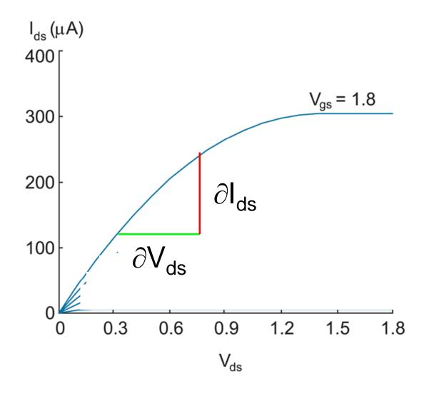
Slope of a curve gives conductance, inverse of which is resistance.
