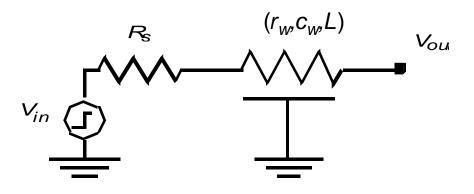
$$\tau_D = R_s C_w + \frac{R_w C_w}{2} = R_s C_w + 0.5 r_w c_w L^2$$
