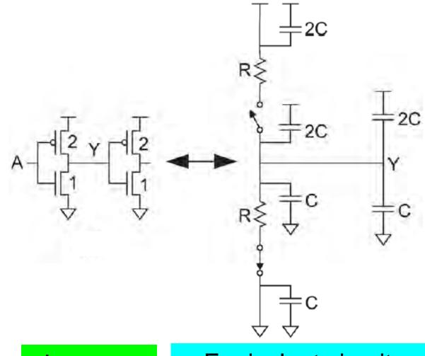
Estimation of delay of a fanoutof-1 inverter.
