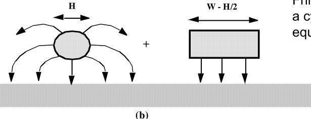
Fringing capacitance is modeled by a cylindrical wire with a diameter equal to the thickness of the wire.
