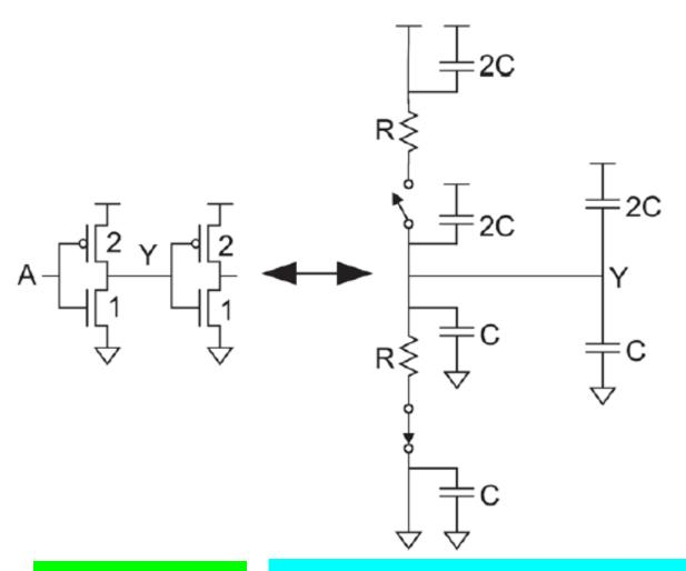
**Estimation** delay of a fanoutof-1 inverter.
