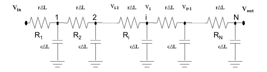
Elmore delay of node  $i: \tau_i = R_1C_1 + (R_1+R_2)C_2 + ... + (R_1+R_2+...+R_i)C_i$
