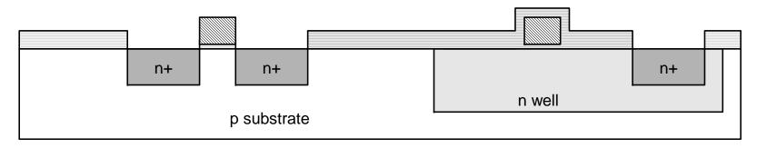
Strip off oxide to complete patterning step
