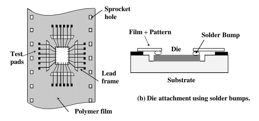
(a) Polymer Tape with imprinted wiring pattern.
