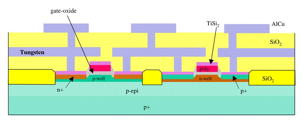
**Dual-Well Trench-Isolated CMOS Process**
